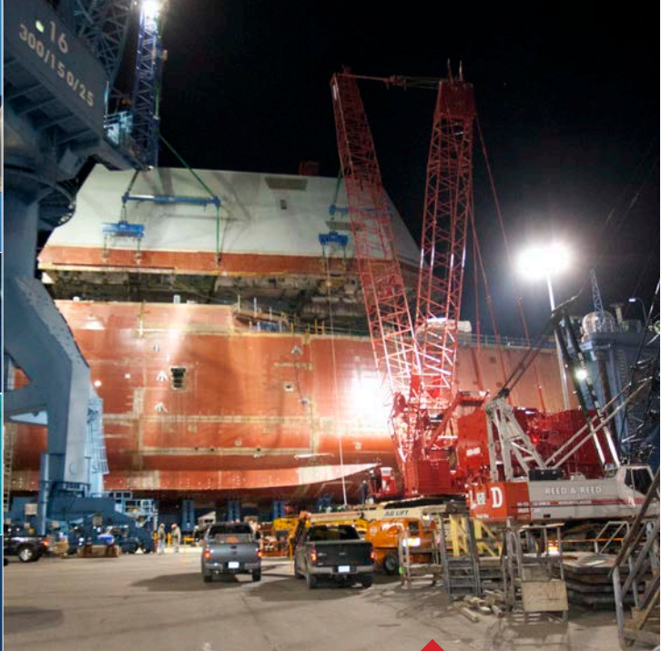
Deckhouse of USS Zumwalt being installed at General Dynamics Bath Iron Works.
